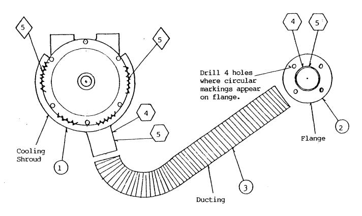
Note: Shroud must be centered on the pump. On some installations the pump may have to be rotated on the mounting pad because of interference with other objects.
